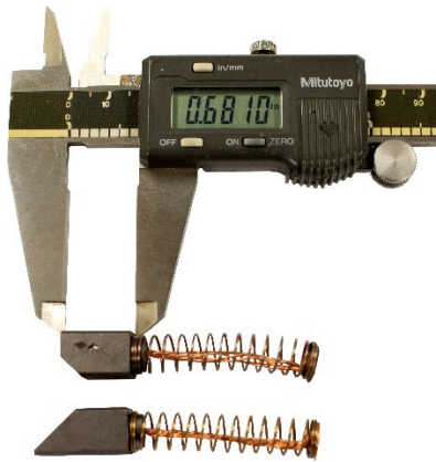
SGS™ CR Series model brush wear after nearly 5 years of continuous run time. Plenty of brush left.
