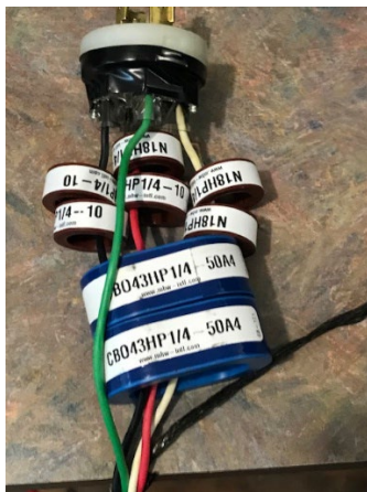
Induction absorbers installed per manufacturer's instructions.
