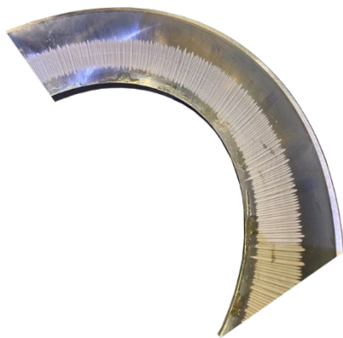
Figure 3: Washboard fluting pattern from a water treatment plant
